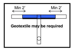
2. For patches in asphalt, a tack coat shall be applied to all edges of the existing asphalt before placing the new pavement. After placing the new asphalt, all seams (joints) between the new and existing pavements shall be sealed with an asphalt tack coat or rubberized crack seal material.
