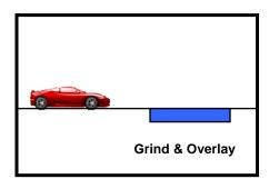
iii. Surface tolerances for street repairs should meet the standard for new construction. That is, the finished surface of the street repair, when tested with a ten (10) foot straightedge parallel to the centerline or perpendicular across joints, will show variations measured from the testing face of the straightedge to the surface of the street repair which do not exceed one quarter (1/4) inch.
