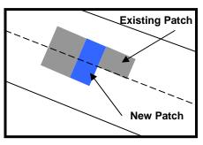
3. Asphalt and concrete pavements should be removed by saw cutting or grinding. Avoid breaking the edges of the existing pavement or damaging the remaining pavement with heavy construction equipment.
