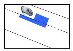
2. Avoid patches within existing patches. If this cannot be avoided, make the boundaries of the patches coincide.
